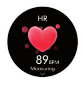
Upon entering the function, the heart rate measurement will start automatically. Wait about 30-60 seconds for the measurement to finish and the result will be displayed. Slide up to see a graph with the heart rate tests results of the current day. On the app you can check the historical data.
