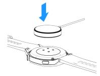
and the smartwatch are properly connected while charging. Do not charge if the watch has water (or sweat) to avoid short circuits and damaging the product.
