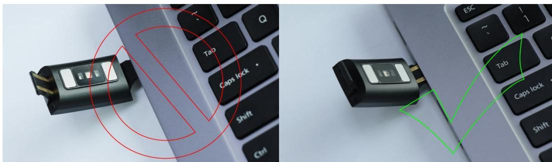
**\*Please be aware that the two contacts of charging cannot contact the conductor at the same time, or it may cause the burning of circuit.**
